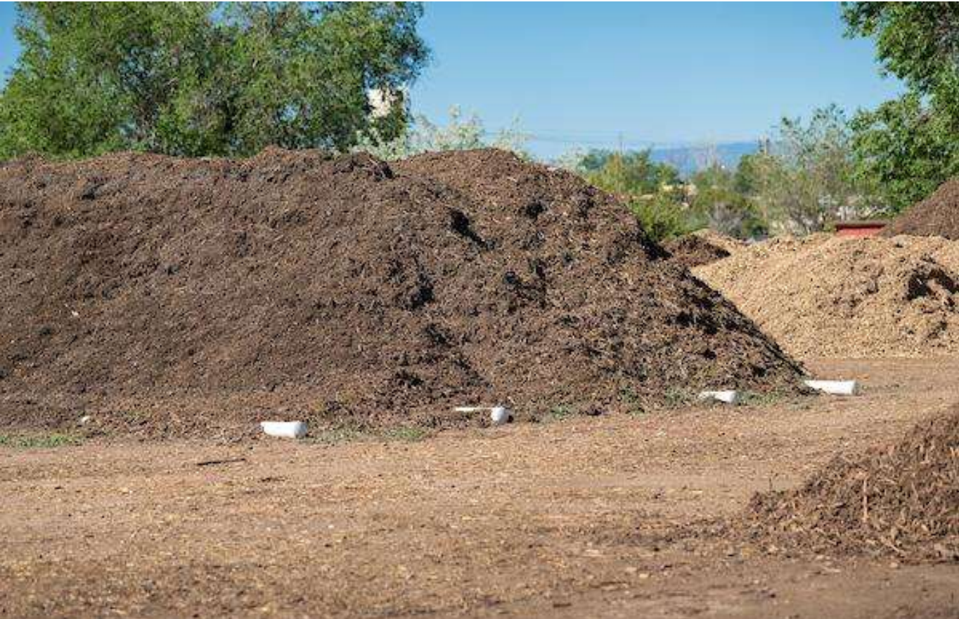
Aerated Static Pile Composting; 5 million pounds of food+wood waste/year on one acre
