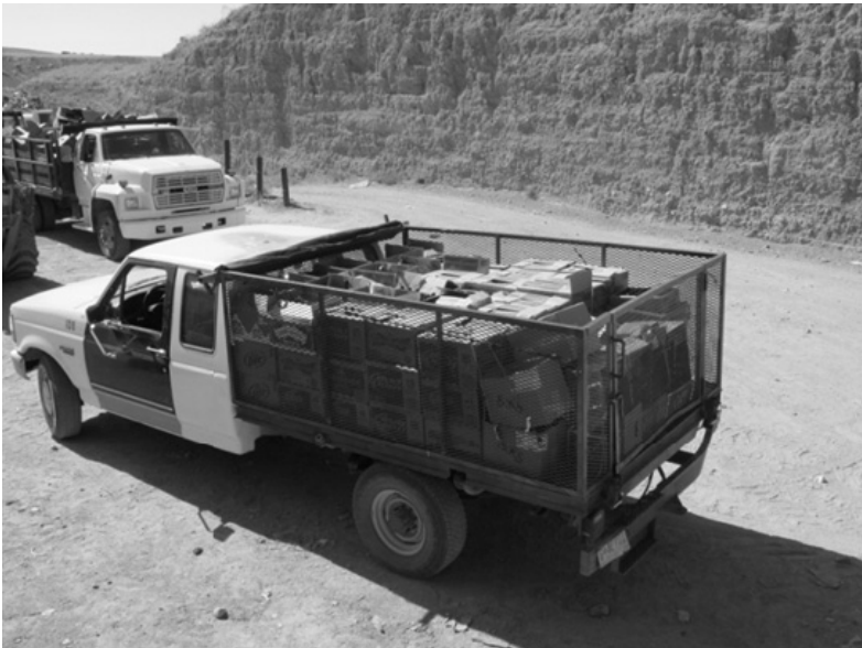
Flat bed truck used to collect glass from commercial sources (bars, restaurants and clubs). Photo courtesy Southwest Solid Waste Authority.
